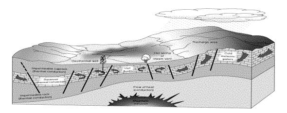
Geothermal energy is harnessed through the utilization of the "kettle concept." The concept is illustrated by Raul C. Sabularse of the Department of Science and Technology, as illustrated by the following diagram:<sup>48</sup>
